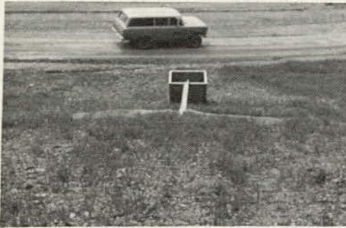
Figure 1. In demonstration No. 2, runoff from 1,000-sq ft subplot is channeled into the collection box to measure sediment yield.
