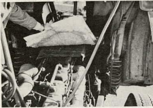
Figure 3. Insulation placed under truck cab.
