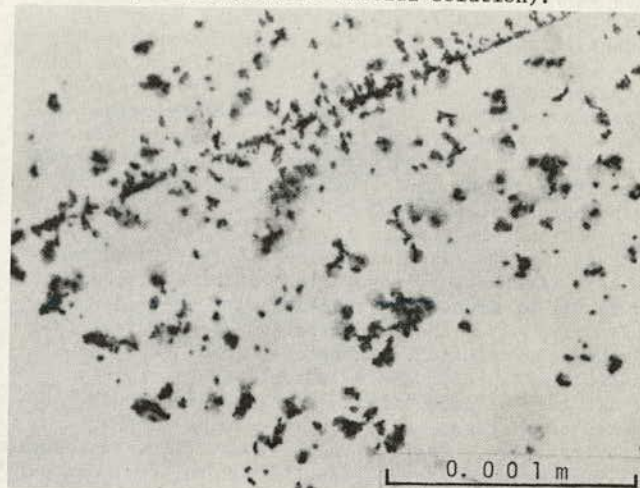
Figure 10. \text{AgNO}_3 replica of a brass substrate surface taken immediately after the removal of a KCl-ice specimen (0.7% in initial solution).
