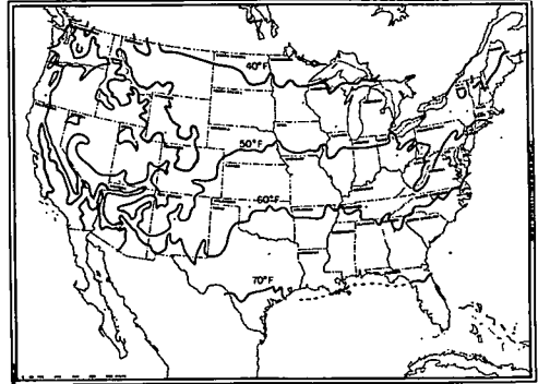
Figure 1. Approximate Distribution of Deep Ground Isothermal Temperatures Based on Mean Annual Temperatures Degrees Fahrenheit. At levels 15 to 30 ft. below the surface, temperatures as shown remain constant and relatively unaffected by variations in atmospheric temperatures throughout the year. At levels above the isothermal zone stored heat from the previous summer tends to inhibit the cooling and freezing of the ground.
