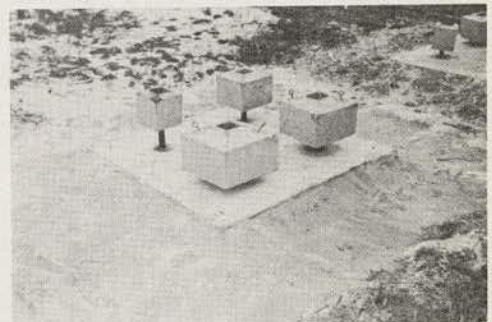
Figure 5. Concrete Slab and Weighted Plungers.
