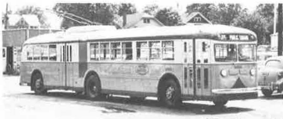
In 1939, the Twin Coach Company built this semi-articulated trolley bus, which bent in the vertical direction only (photograph courtesy of Flxible).
