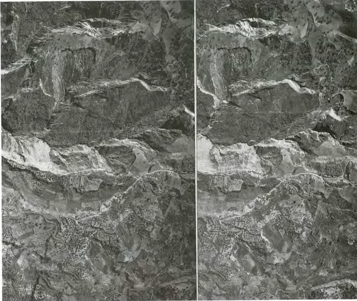
FIGURE 8-4 Translational slides controlled by dip slopes in sequence of very friable sandstones alternating with siltstones and mudstones. Joint-controlled back scarp, linear patterns, and micromorphology of area where the sandstones have slid away ( lower part ) are diagnostic for landslides. Somewhat comparable morphology and change in land use ( upper part ) are indicative of landslides that have rapidly transformed into earth flow because of higher clay content (original photograph scale 1:17,000, Basilicata, Italy).
