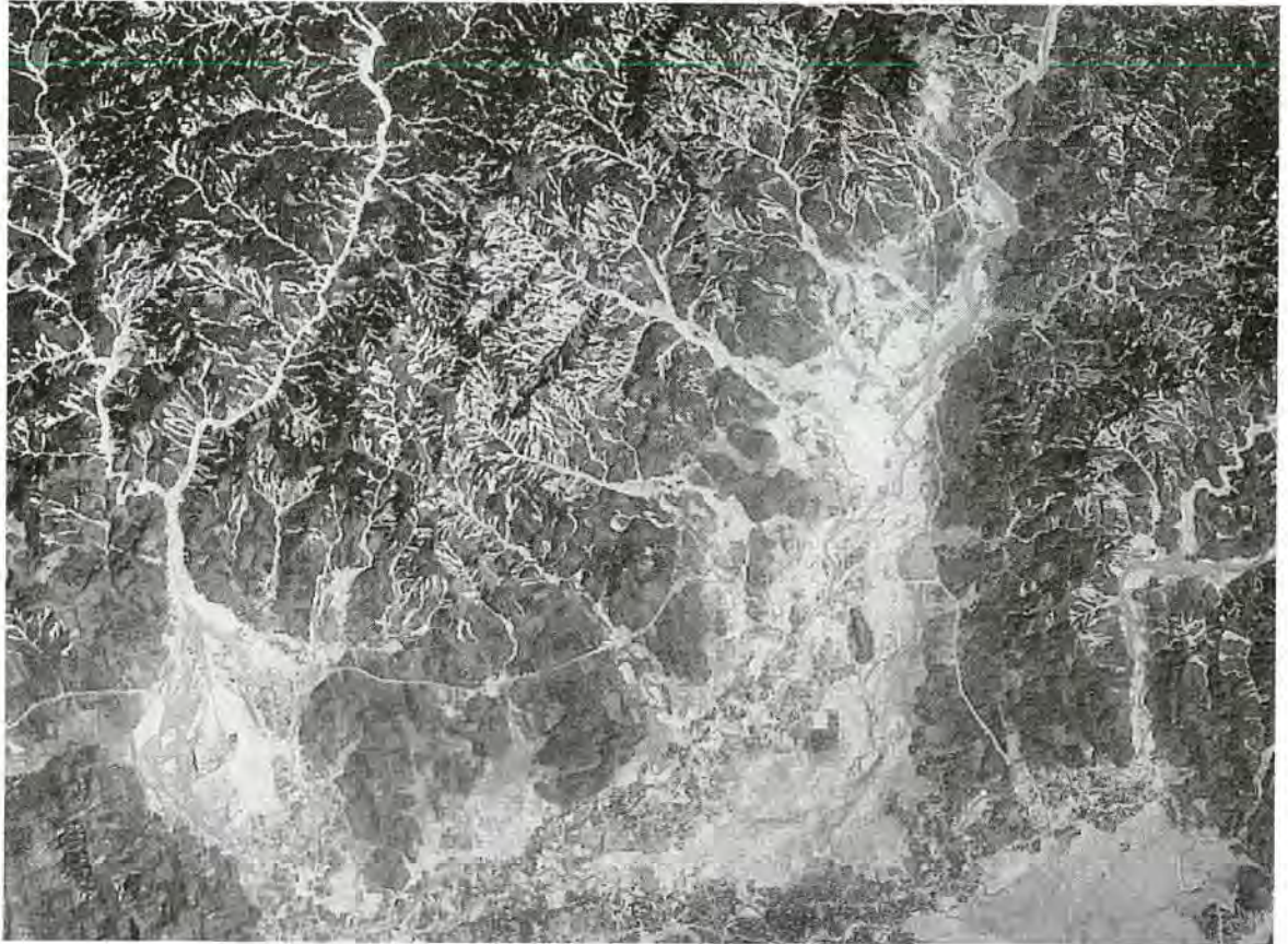
FIGURE 8-7 SPOT multispectral satellite image with relatively good spatial resolution can be used profitably in assessment of areas affected by slope movements. Example shows area in Thailand where large number of shallow debris slides generated large debris flow that traveled through valleys, damaging agricultural fields and houses.
