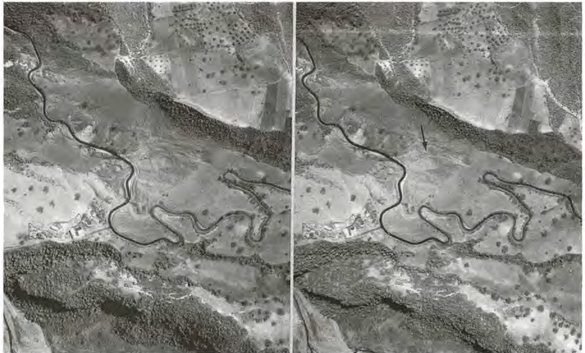
FIGURE 8-2 Faint tonal and textural differences characterizing surficial mud slides in marly clays. Slope failures can be readily interpreted when stereogram is viewed with pocket stereoscope. Although these mass movements are significant because they frequently damage roads, their size precludes them from being interpreted on smaller-scale images (original photograph scale 1:17,000, Basilicata, Italy).
