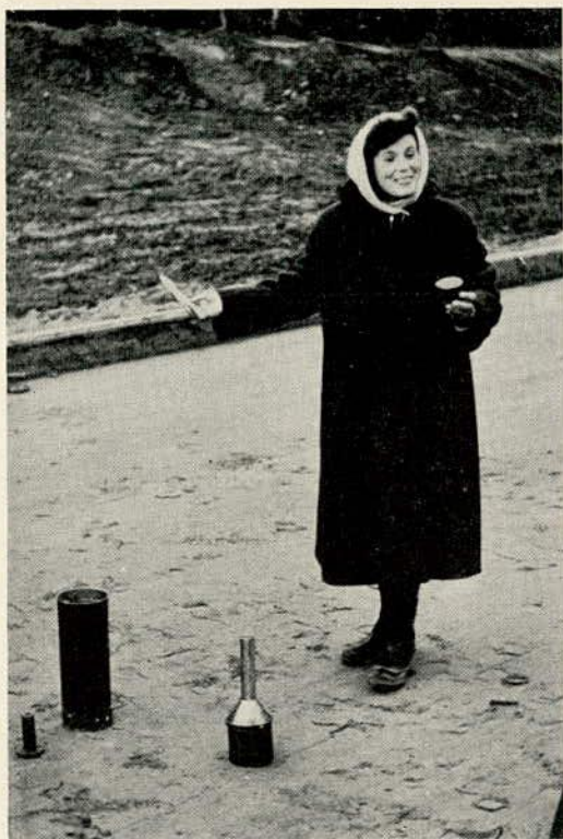
FIGURE 15 Density test on compacted subbase.
