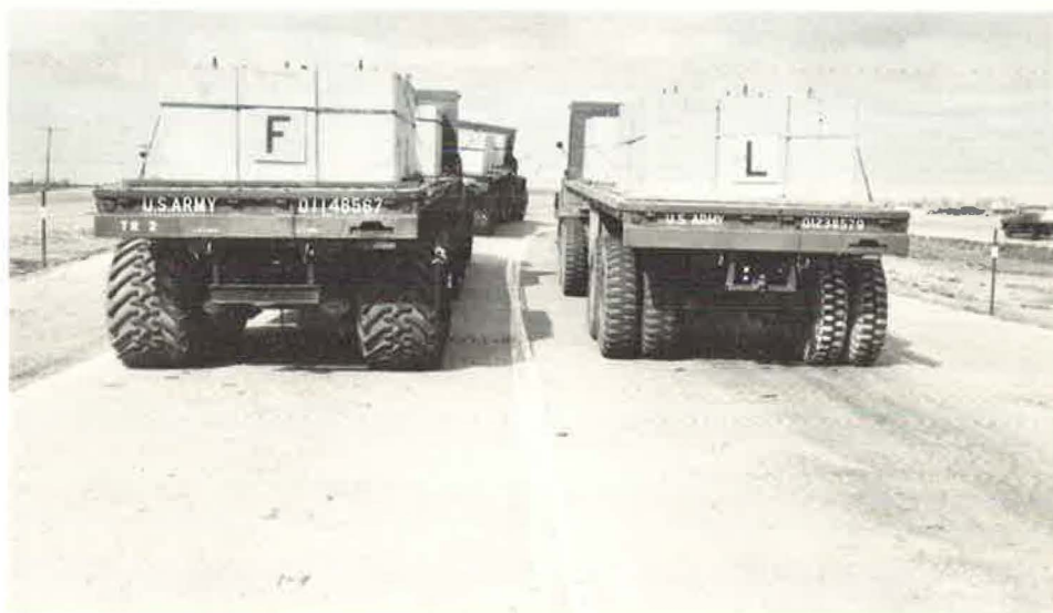
Figure 52. M-52 tractor-semitrailers equipped with LPLS tires (left) and conventional tires (right).
