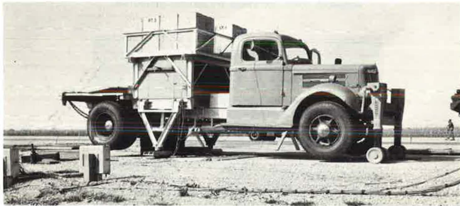
Figure 39. Truck-mounted vibrating loader. Load was transmitted to pavement through inverted A-frames and wooden pads. Front tires were lifted from pavement to minimize vibration at front axle.
