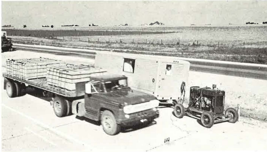
Figure 35. Instrument van taking dynamic measurements. Device on pavement just ahead of truck measures transverse placement.
