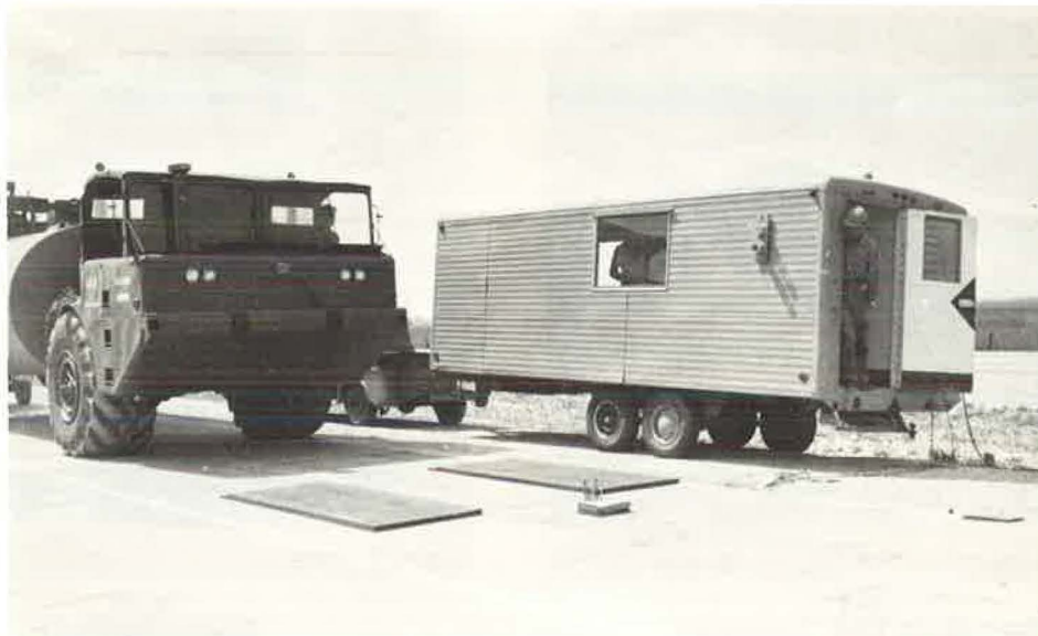
Figure 54. GOER operated over ramps in drop tests at rigid pavement instrumentation van.
