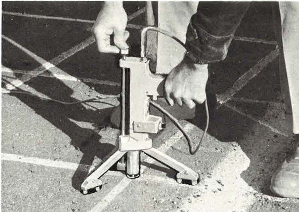
Figure 24. Electrical device used to measure vertical movement of pavement.
