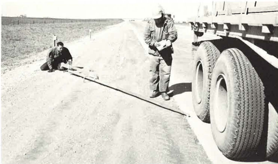
Figure 37. Measuring static rebound deflection with the Benkelman beam.
