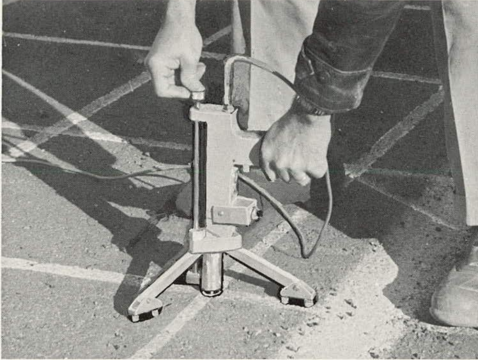
Figure 40. Electrical device used to measure vertical movement of pavement.
