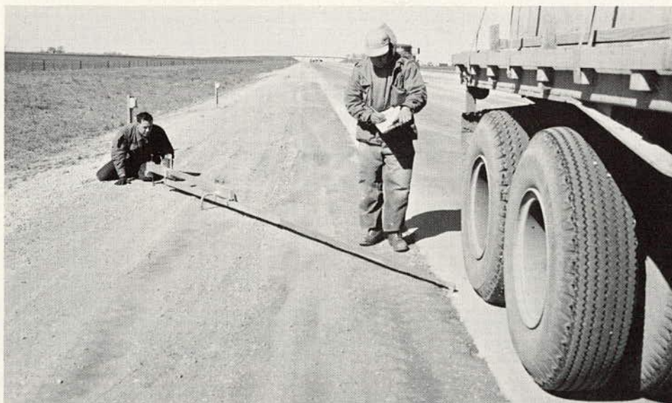
Figure 146. Measuring static rebound deflection with the Benkelman beam.
