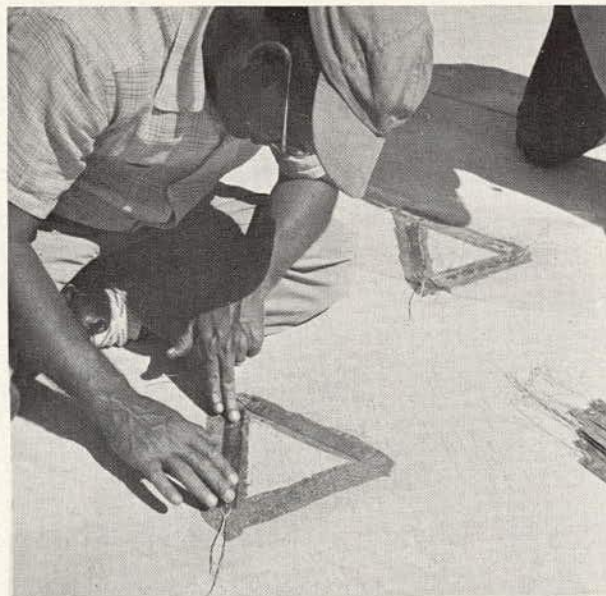
Figure 183. Two of the several steps in installation of strain gages in Loop 1.
