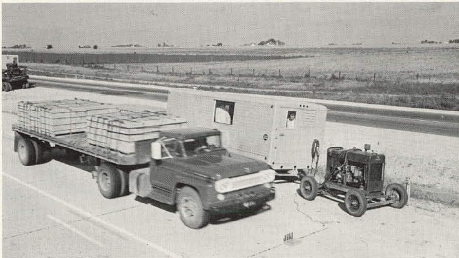
Figure 141. Instrument van taking dynamic measurements. Device on pavement just ahead of truck measures transverse placement.
