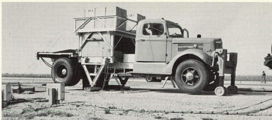
Figure 185. Truck-mounted vibrating loader. Load was transmitted to pavement through inverted A-frames and wooden pads. Front tires were lifted from pavement to minimize vibration at front axle.
