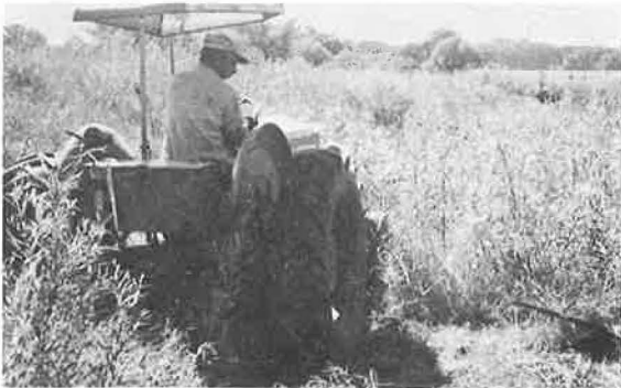
Figure 29. Tractor with 6' sickle bar mower cutting high weeds on ROW.
