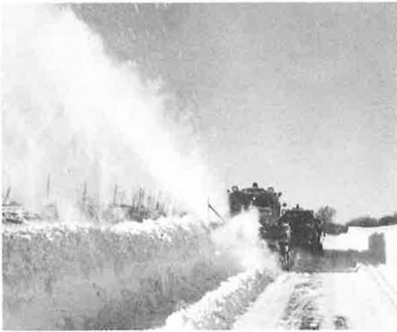
Figure 34. Heavy duty truck with rotary plow removing drift on roadway surface.
