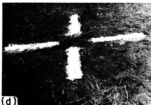
Figure 7. Some targets used for placement on markers of control points in Kansas research projects to determine a good material and proper procedure for setting targets. (a) Very rough X limed target marker; target used with good success; open cross, however, better target. (b) Typical target made of canvas, using four strips. Two strips may be used, however, by darkening center portion with dirt or paint. (c) Typical closed cross constructed of lime by using care in placing lime to general size and shape suggested for photography taken from a flight height 1,500 ft. (d) Typical open center cross made of lime and having same characteristics as closed cross. This cross seems to have best characteristics for pass points at which elevation is measured for leveling stereoscopic models.
