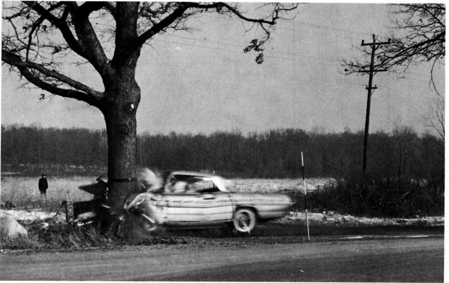
Figure 4. Car-tree impact—64 mph.
