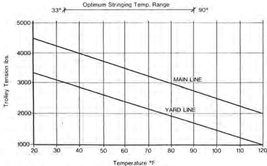
FIGURE 23 Tension and temperature chart for 4/0 trolley.
