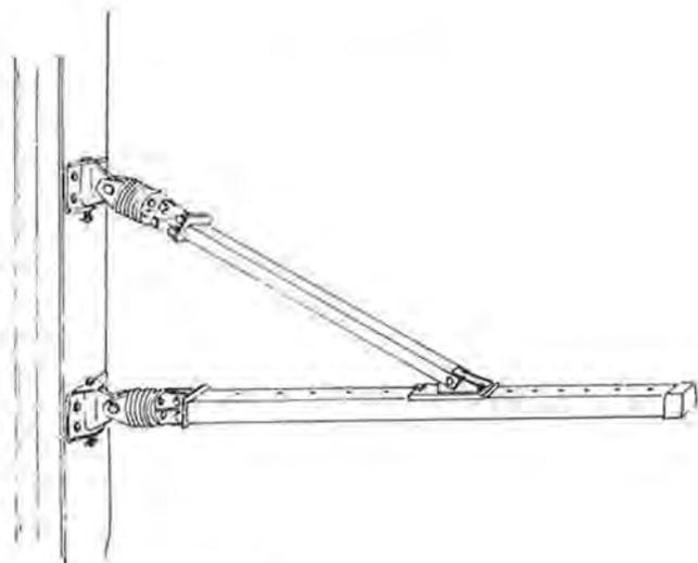
FIGURE 12 Bracket tubes.
