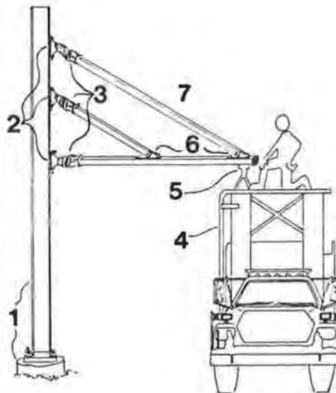
FIGURE 18 Bracket installation.
