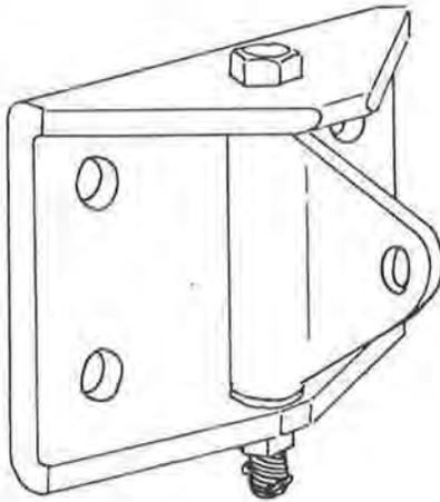
FIGURE 14 Bracket hinge.
