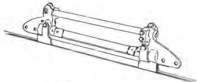
FIGURE 7 Section insulator.
