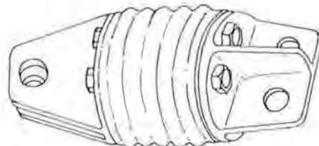
FIGURE 11 Bracket insulator.
