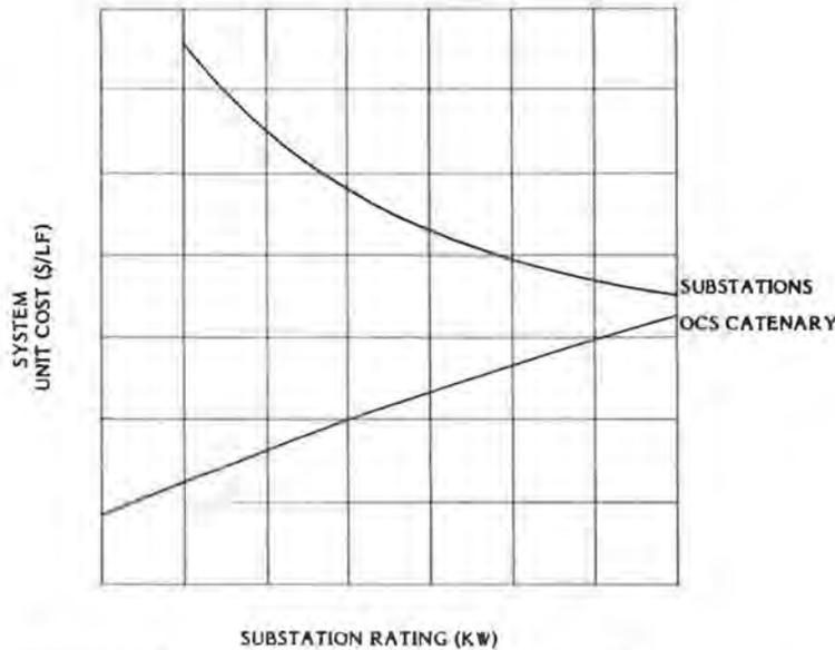
FIGURE 3 Traction electrification system unit cost curves.
