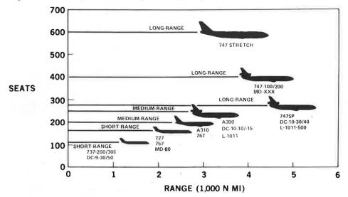
aircraft with a capacity approaching 600 seats. In between are the twin and tri-jet narrow body and tri-jet wide body aircraft having from 150 to 300 seats.
