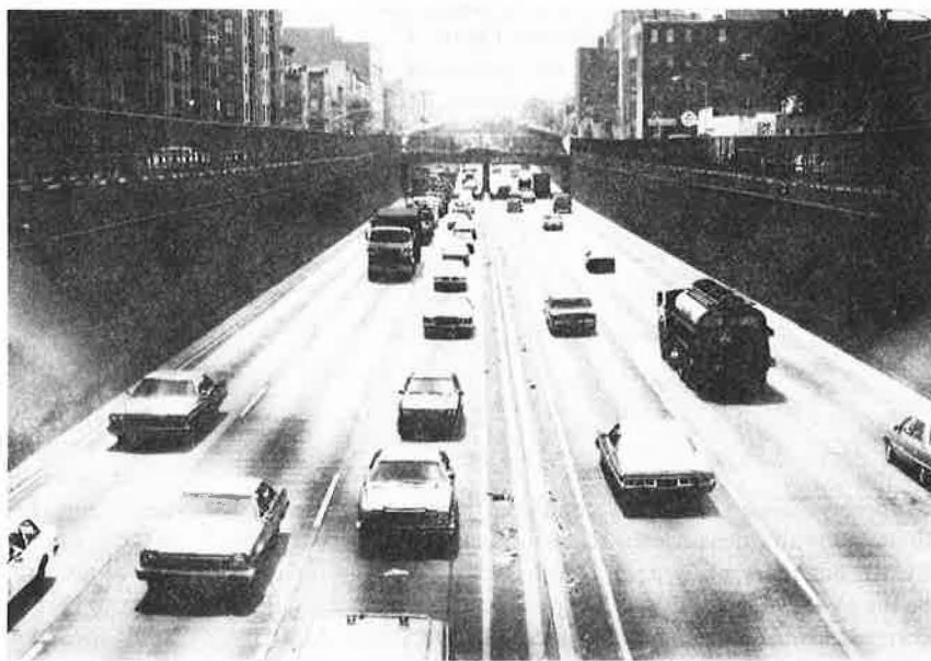
Illustration 3-4. Large gaps in front of trucks or other heavy vehicles are often unavoidable even on relatively level terrain.
