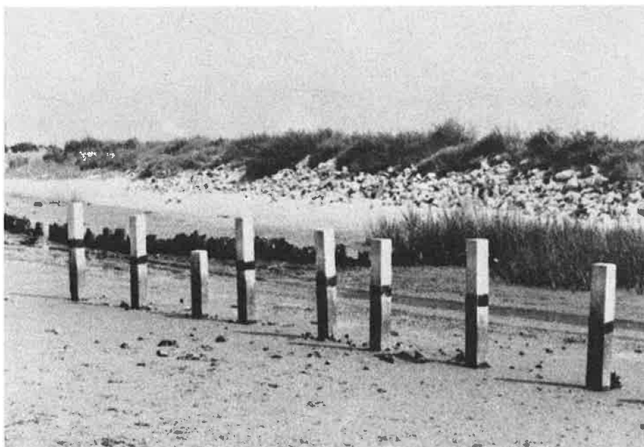
Figure 4 Matanzas Inlet test site after placement of test pilings in 1979 with application of coal-tar epoxy bands around areas containing the rebar support chairs.
