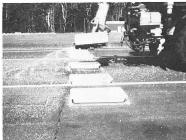
Figure 1 Pans laid in rows normal to direction of truck travel to catch salt leaving the spinner.
