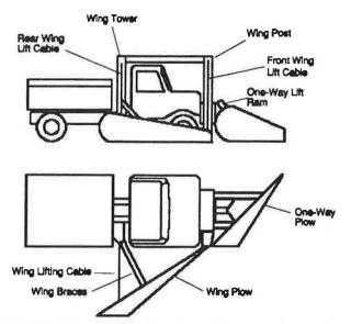
FIGURE 1 Top and side views of a snow plow and wing plow vehicle.
