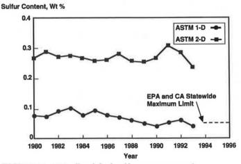
FIGURE 1 U.S. diesel fuel sulfur content trends.
