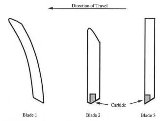
FIGURE 2 Cutting edges used in experimental study.
