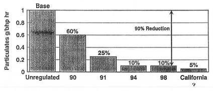
Model Year FIGURE 2 EPA Heavy-Duty Truck engine PM emission standards.
