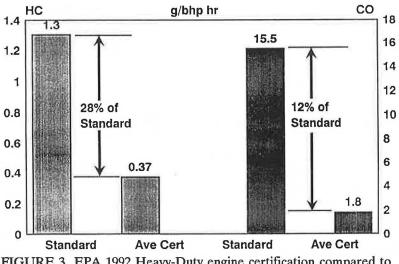
FIGURE 3 EPA 1992 Heavy-Duty engine certification compared to emission standards.
