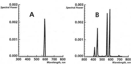
FIGURE 2 Spectral power distribution of various light sources: A) Low pressure sodium, and B) Clear Mercury.
