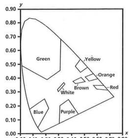
0.00 0.10 0.20 0.30 0.40 0.50 0.60 0.70 0.80 FIGURE 6 Chromaticity regions specified by the CIE for ordinary colors under D65, daylight (3). The CIE Tristimulus Values are x and y. Following the perimeter changes hue and saturation changes from center to outer edges.
