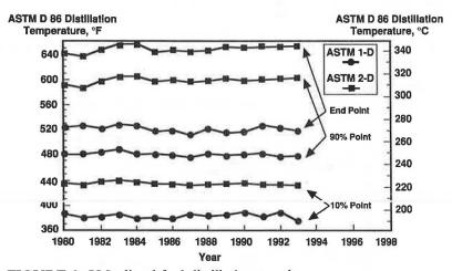
FIGURE 3 U.S. diesel fuel distillation trends.
