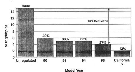
FIGURE 1 EPA Heavy-Duty Truck engine NOx emission standards.
