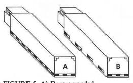
FIGURE 5 A) Recommended configuration of retroreflective materials, and B) optional treatment with gaps on sides. (2)
