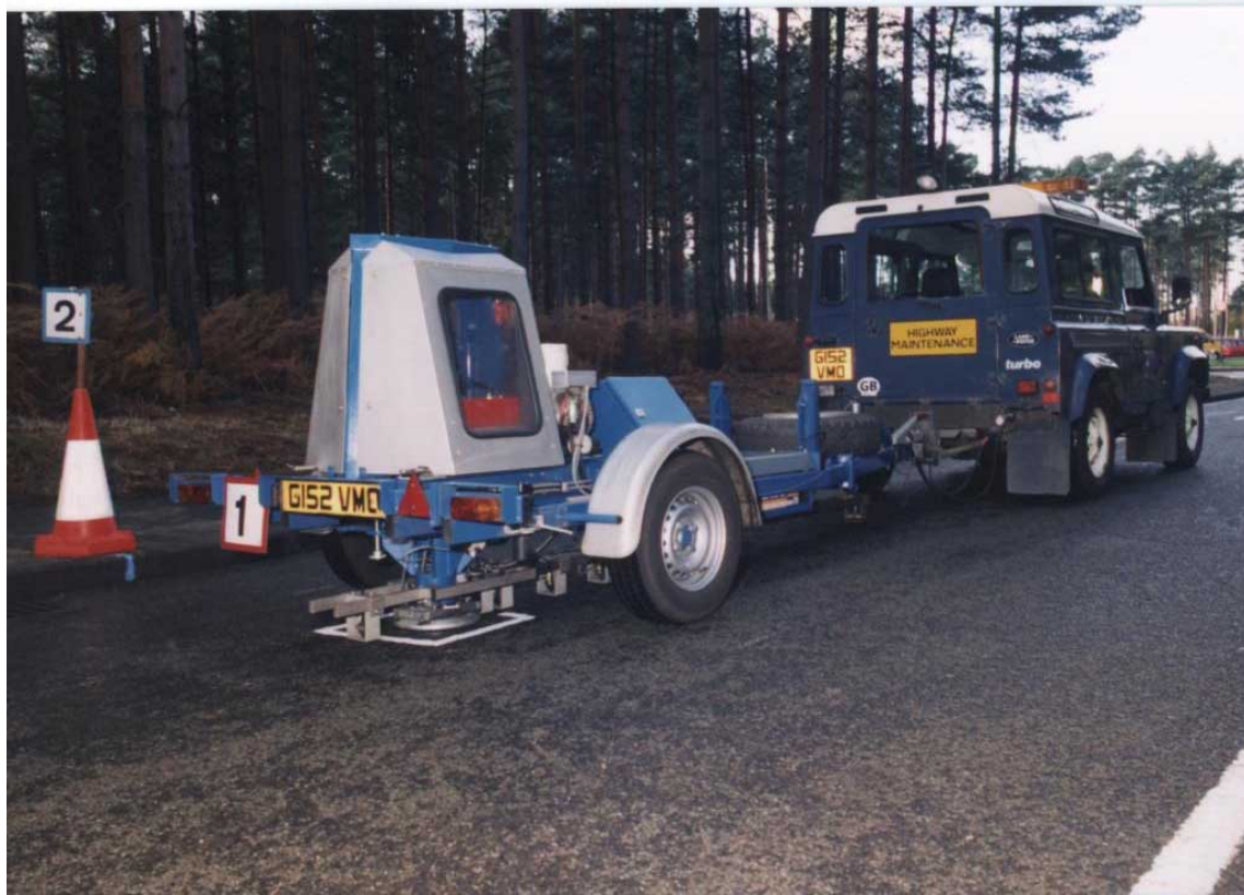
FIGURE 7 FWD carrying out measurements.
