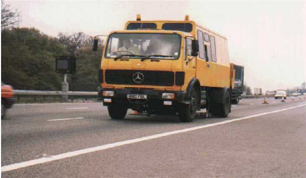
FIGURE 5 Deflectograph survey in progress.
