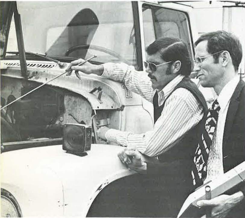
6 The noise level from a stationary truck motor is measured by Peter Renz (left) and Larry D. Pope.
