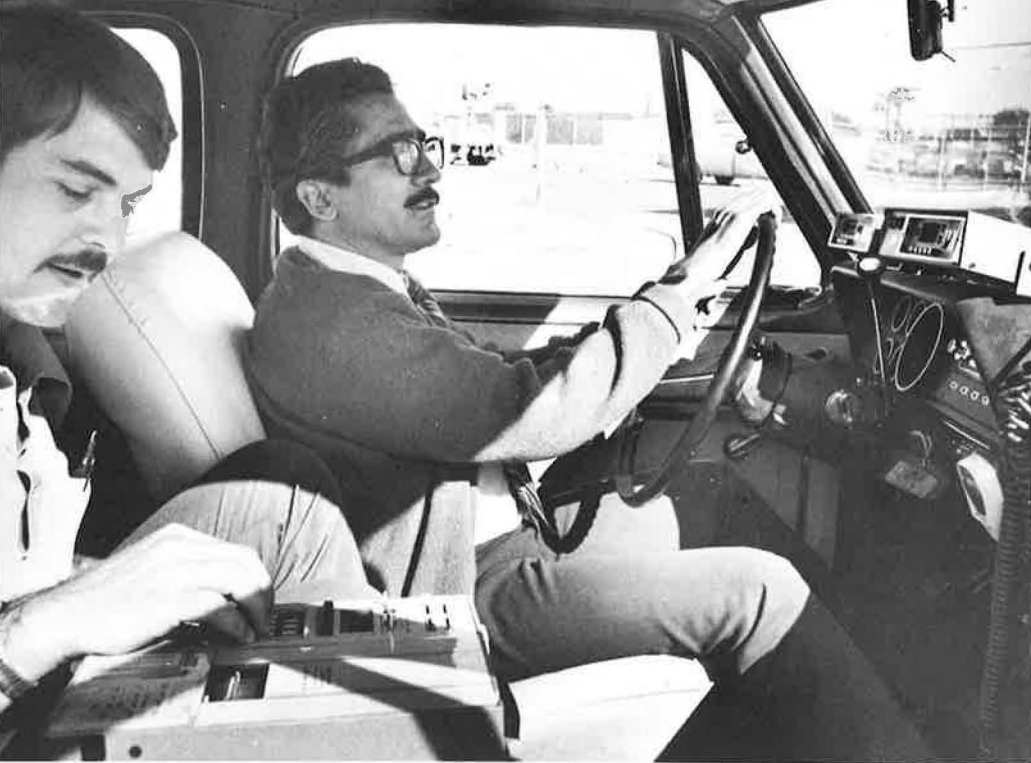
1 Author David Olivarez is driving while Kohn Blackledge operates the printer to record no-passing-zone data. The distance-measuring and range-tracking instruments can be seen on the dashboard.
