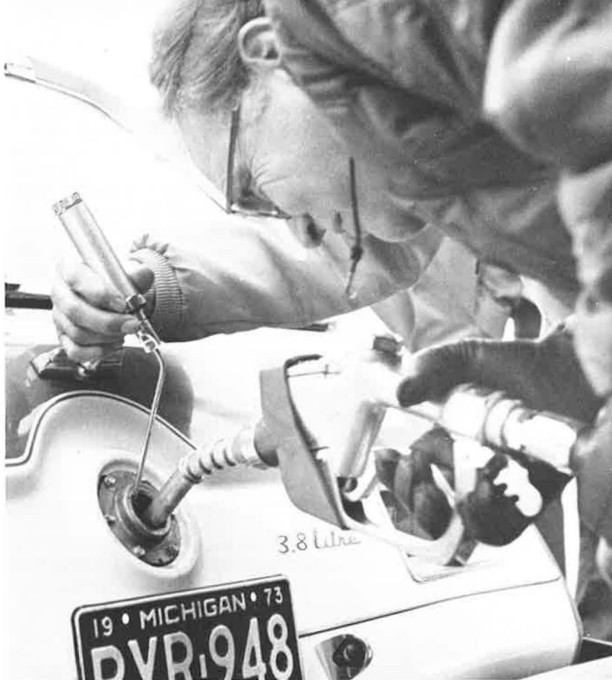
In 1 of 3 Collegiate Economy Runs sponsored by the American Motors Corporation during 1974, the winning 6-cylinder Gremlin covered 25.29 miles per gallon. Here an official takes the temperature of the gasoline before the start to permit measuring fuel accurately by volume regardless of expansion or contraction caused by outside temperature variations.
