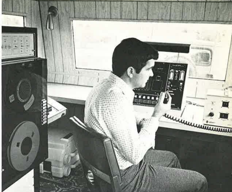
James Burt, a researcher with the Louisiana Department of Highways, tests a computerized system that weighs trucks while they are moving at normal highway speeds. The trucks are weighed by the use of metal load plates, which are placed in the surface of the highway and are connected by wires to the computerized equipment in a trailer by the roadside. Burt is radioing a permanent highway department weighing station about 5 miles (8 km) away to have the computer's data compared with the weight taken at the station. He served as co-principal investigator for a recently concluded project to test the equipment
