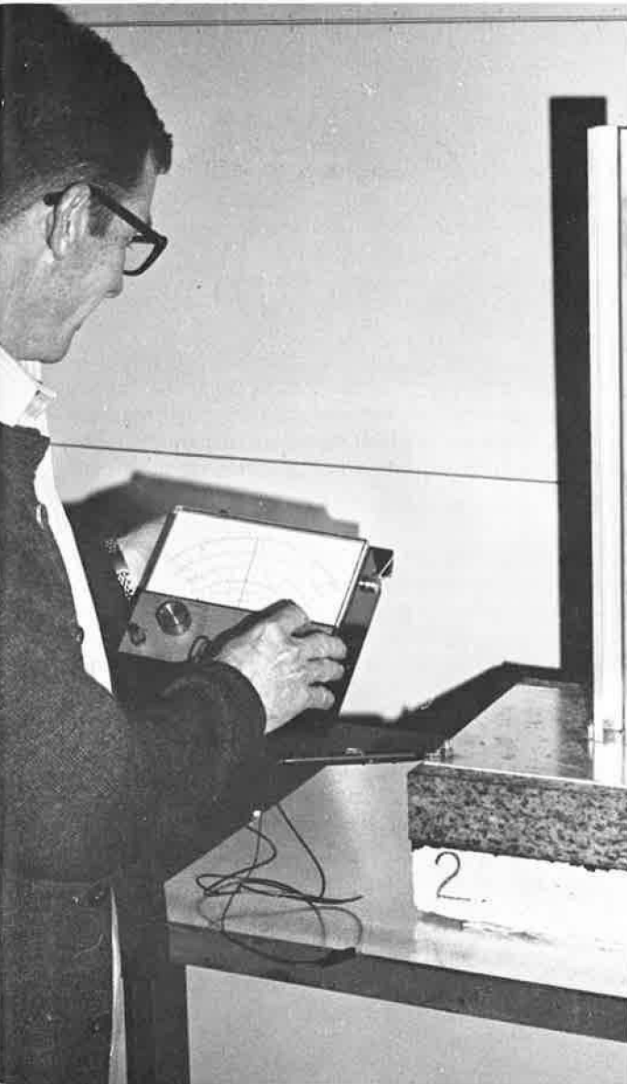
A research technician operates the conductivity test apparatus used to evaluate bridge deck waterproofing membrane systems in the laboratory of the Washington State Department of Highways.
