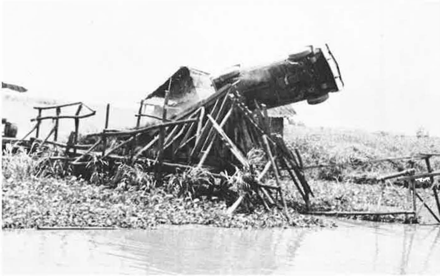
Driver Lauren Willert crosses a Thailand river in an unconventional manner during a chase scene from the latest James Bond film, The Man With the Golden Gun. The configuration of the ramps at either end and the computation of speed, vehicle weight, and other factors were determined by Calspan Corporation using a sophisticated computer program. The ramps look flimsy, but are actually rigidly constructed of teakwood.
