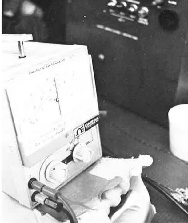
An electric thermometer, attached by thermocouples to the treated portion of the deck, was used to record temperature readings during the heating process.
