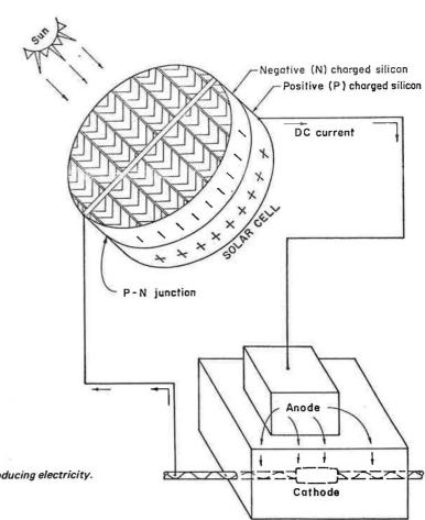
Figure 1. Solar cell producing electricity.
