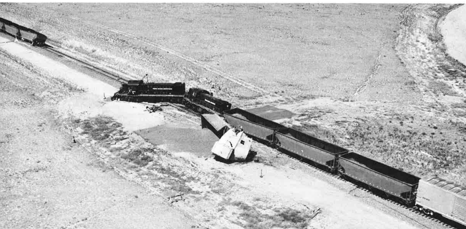
Results of a locomotive/caboose test. The caboose traveled up and over the hopper car.
