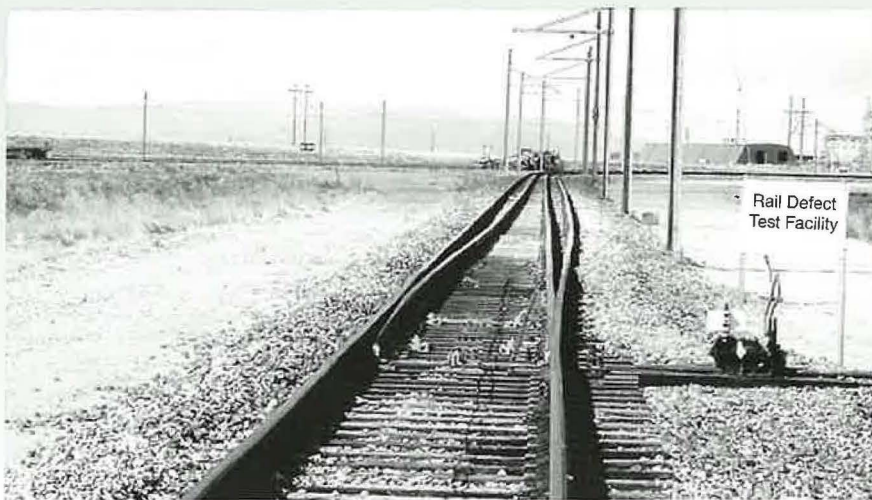
FIGURE 3 Performance evaluation of state-of-the-art rail detector cars at Transportation Technology Center's Rail Defect Test Facility will improve reliability and accuracy of internal rail defect inspection.
