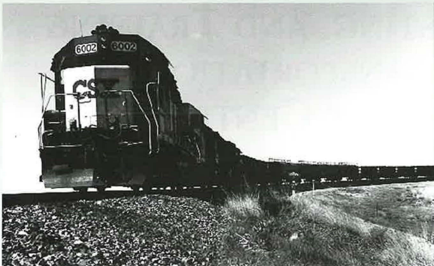
FIGURE 2 Track performance under 39-ton, heavy-axle loads is measured at Transportation Technology Center's Facility for Accelerated Service Testing to determine safety and performance benefits of improved suspension trucks.
