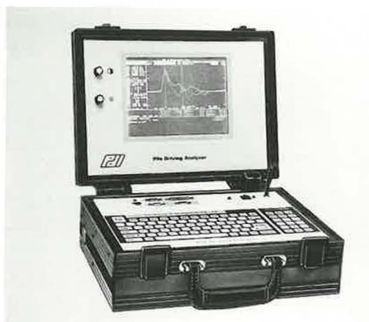
FIGURE 3 Pile driving analyzer.
