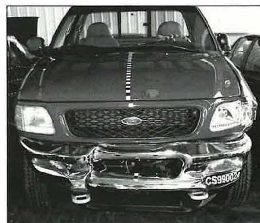
FIGURE 6 Stiff tow hooks below bumper of the Ford F-150 4x4 pickup probably reduced risk of chest injury in the Mercury Grand Marquis by accelerating the struck driver's pelvis earlier than the chest. Paint transferred to leading edge of hood shows where the dummy's head contacted hood during test.
