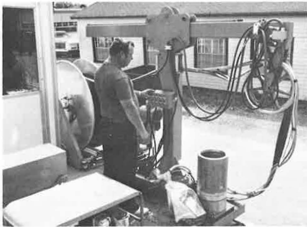
Different view of extendible arm with hydraulic controls and diving bell disassembled.
