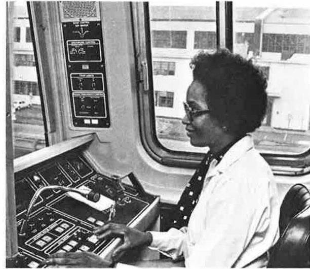
Automatic train control system simplifies duties of operator, who can override system in an emergency.
