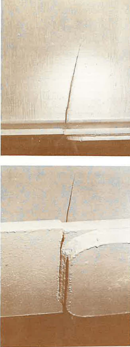
5. Side view (top) of a cover-plated steel girder shows a fatigue crack starting in the flange at the toe of a fillet weld at the end of the cover plate and extending through part of the web. The same girder (bottom) is viewed from below showing fatigue crack extending through the flange (foreground) and into the web (top of picture).
