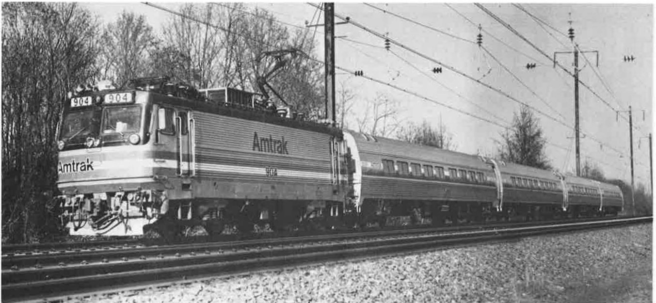
An Amtrak Express Metroliner, powered by an AEM-7 high-speed electric locomotive and equipped with new Amfleet II cars, dashes toward Washington on its way from New York. Amfleet II cars can be distinguished from the original Amfleet equipment by their larger windows and vestibules located in only one end of the car. (Amtrak photo)
