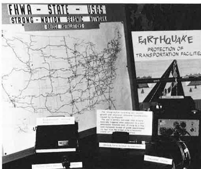
Field measurements of ground motions and structural response during earthquakes provide necessary linkage between the results of laboratory tests, analytical modeling, and actual seismic events. Strong-motion recording units have been installed on bridges in six states as part of a cooperative program involving FHWA, the U.S. Geological Survey, and various state highway agencies.
