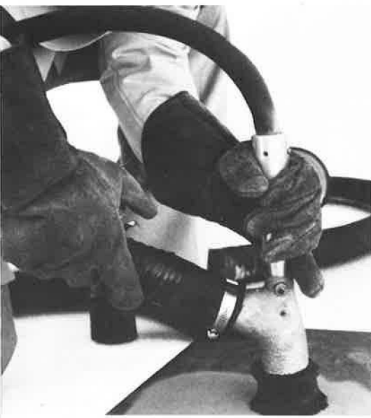
Vacuum blaster in operation (photograph from Vac-U-Blast International).
