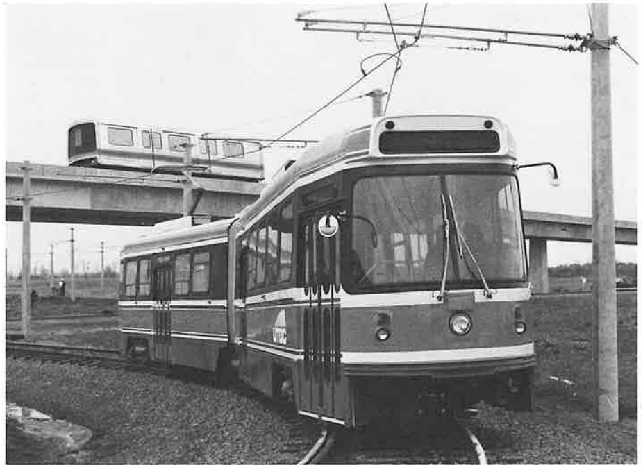
Articulated LRV developed by UTDC/Hawker Siddely at the company's Kingston, Ontario, Canada, research facility. LRVs to be manufactured for Toronto, Canada, and Santa Clara County (San Jose), California, will be based on the design of this car.
