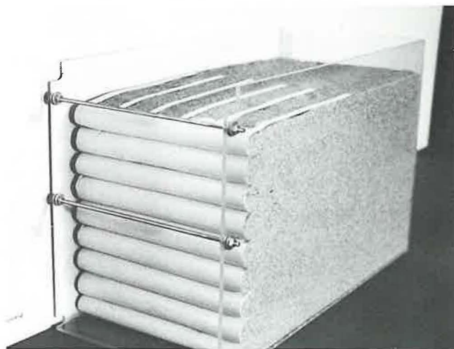
FIGURE 1 Dry sand reinforced with strips of paper.
