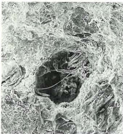
FIGURE 4 Air void in concrete with fibrous halite crystals.
