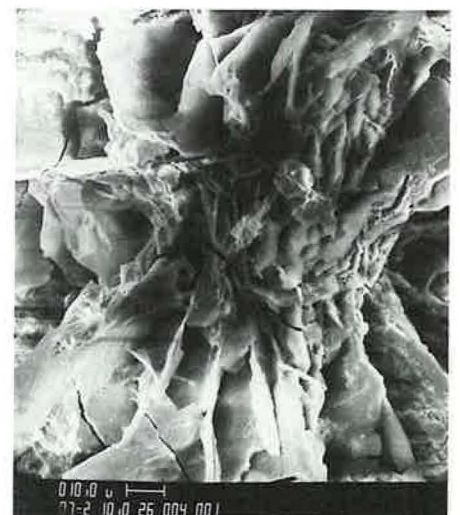
FIGURE 6 Boxwork rust crystals growing within portland cement concrete.
