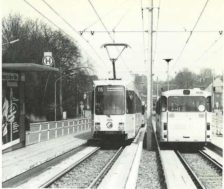
Guided-bus system in Essen, West Germany, mixes operations, increasing corridor capacity and facilitating modal transitions.
