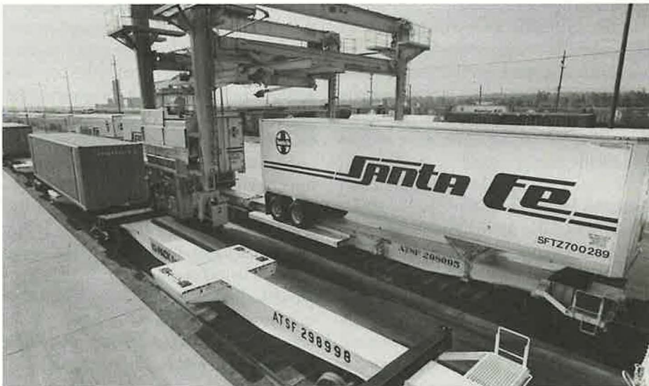
A freight container swings aboard Santa Fe Railway Company's new skeleton-like car that is expected to produce a fuel savings of more than 15 percent compared with conventional equipment. The experimental, articulated car can carry 10 40-ft containers or 20 20-ft containers or a combination of these containers. (photograph from Santa Fe Southern Pacific Corp.)
