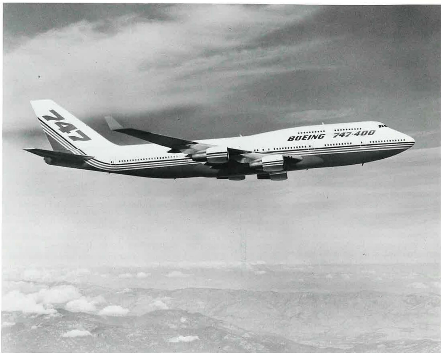
The Boeing 747-400 is the first production commercial airliner to feature winglets as part of the aerodynamic improvements. The airplane uses the same fuselage and basic wing of the 747-300, but has a 6-ft (1.8-m) wing-tip extension in addition to the 6-ft-high winglets.
