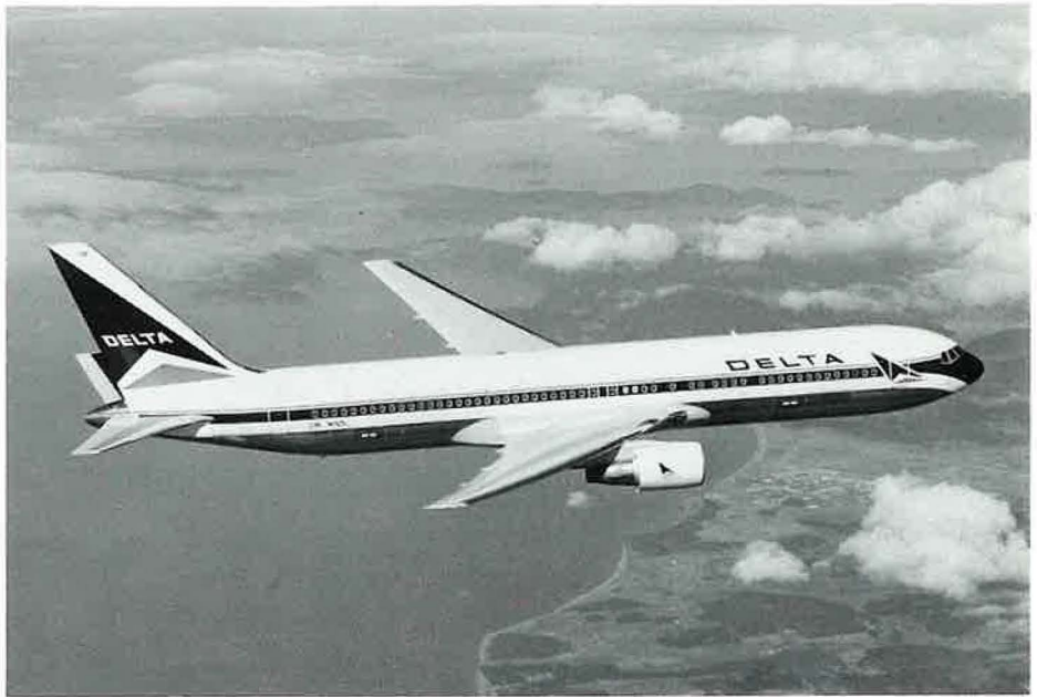
The latest version of the Boeing 767-300 airplane with General Electric CF6-80A2 engines on its maiden flight during a test program of the Delta Airlines ordered model. The medium-range, fuel-efficient, longer aircraft burns 12 percent less fuel per seat than the 767-200 and about 34 percent less than the DC-10.
