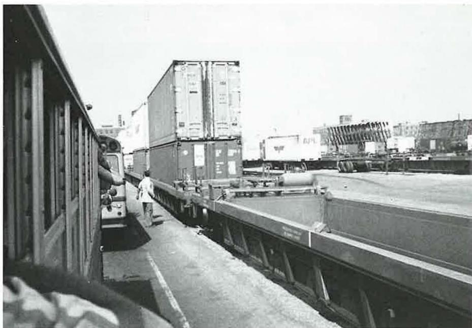
Double-stacked container train at Global One. Containers up to 45 feet long are stacked two high. Low profile and center of gravity provide a smooth ride quality.
