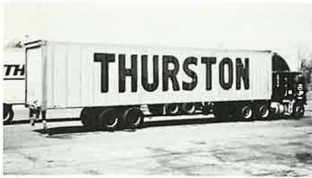
Five-axle tractor-semitrailer, the most important vehicle in the nation's freight truck fleet.
