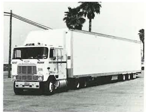
Six-axle semi, with long trailer and low profile tires to allow a lower trailer floor, designed for maximum cargo volume capacity.
