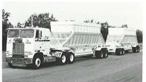
Nine-axle double with trailers each about 32 ft long, used to haul produce and other commodities in several western states. In trailer lengths, axle configuration, and axle loads, the vehicle is similar to the Turner truck concept.
