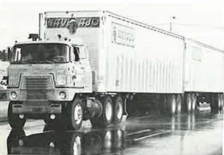
Long, nine-axle double trailer truck, sometimes called a turnpike double. Similar vehicles operate in about 13 states.
