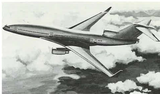
Subsonic airplanes are expected to reach speeds close to Mach 0.95 early in the 21st century compared with jets that now cruise at Mach 0.8. This type of large-bodied aircraft may carry 500 to 600 passengers. (photograph from The Boeing Company)
