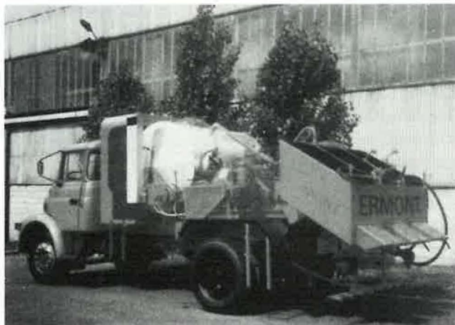
Widely used in France, the patching truck transports personnel, aggregates and bitumen, and the equipment.
