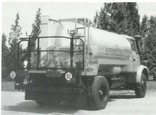
The bitumen distributor carries a tank ranging in capacity from 3,000 to 20,000 liters. The binder (bitumen or bitumen emulsion) is transferred from the tank to the road via a distribution spray bar fed by pressurization of the binder.
