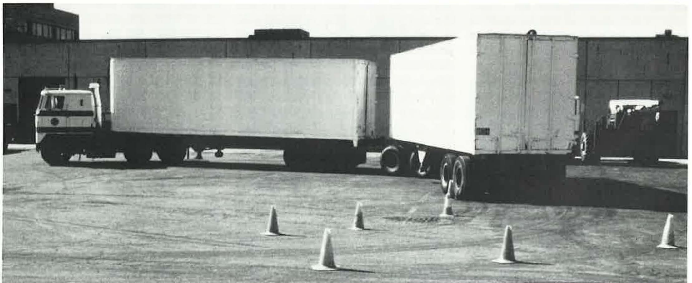
Prototype of one possible Turner truck configuration undergoing a demonstration of cornering ability at the University of Michigan. Analysis of handling and stability of Turner trucks is being performed at the university in support of TRB's Turner Proposal study.
